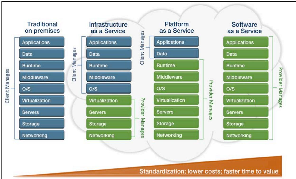
**Figure 1: Application Deployment - Traditional and Cloud-based**
